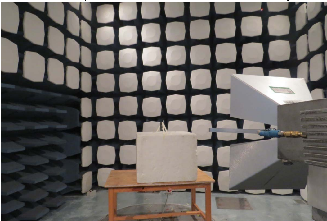
Picture 1: Radiated Spurious Emissions Test setup
