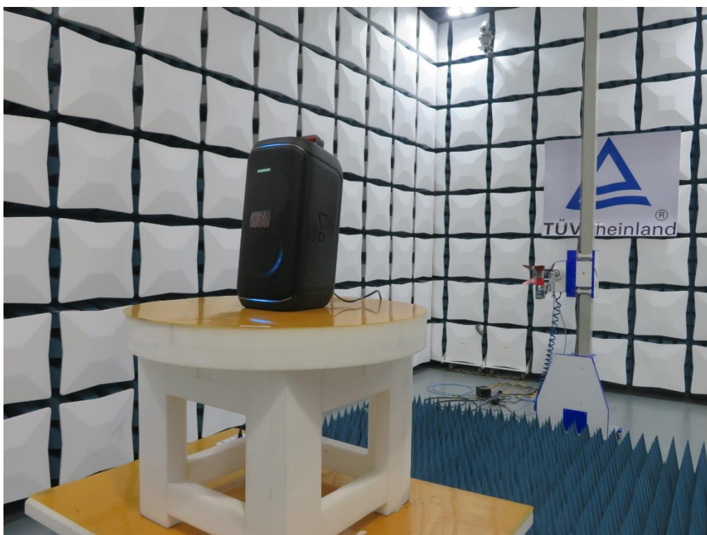
Photograph 2: Set-up for Radiated Spurious Emission, Above 1GHz
