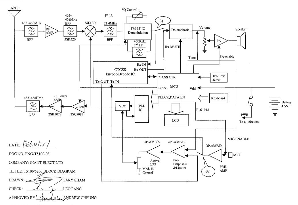
REMARK WHEN S1 AND S2 ARE CLOSED THE SIGANL WILL BE BYPASS CTCSS IC AND REPRESENT MODEL T5100.
