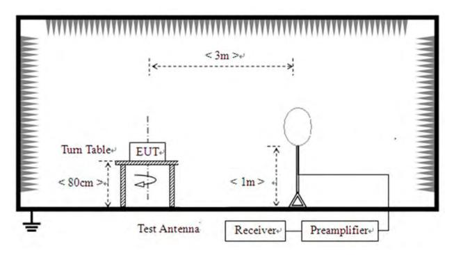
2) For radiated emissions from 30MHz to1GHz
