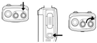
Rotate the channel selector knob to choose the desired channel.
