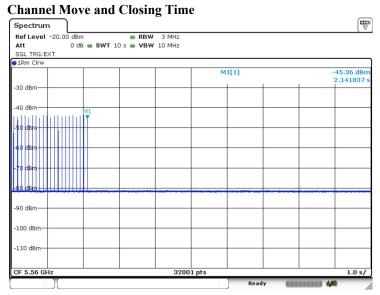
**Channel Closing and Channel Move Time Detailed Results**
