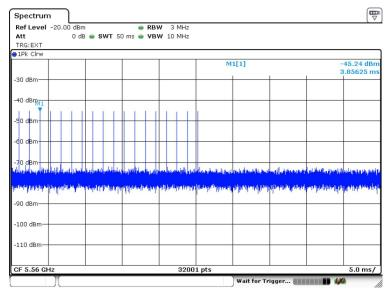
Peak of -45.24dBm, with losses at combiners factoring antenna gain to be 15.81dB, therefore level going into antenna port is -61.05dBm which exceeds threshold level of -64dBm for successful detection.
