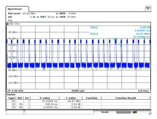
The resulting plot data was extracted and post processed, giving a duty cycle of 26.6%.
