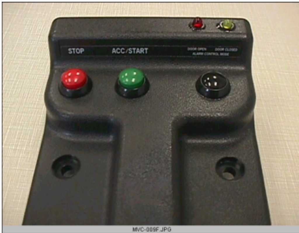
Strattec - Close up of Ignition Reader
