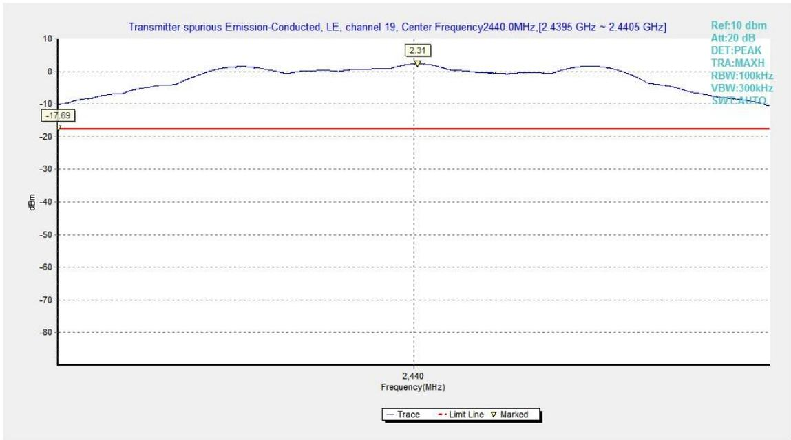
**Fig.10.** Transmitter Spurious Emission - Conducted: GFSK, 2440MHz
