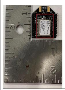
XBee XR 900 with RF-pad output on pin side of module carrier
