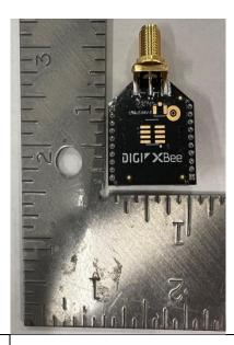
RP-SMA on reverse side of carrier
