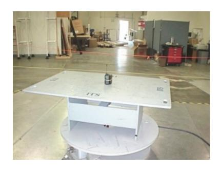
Test Setup – Line Conducted Emission
