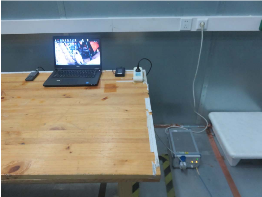
Picture 2 Conducted Emission Test Setup
