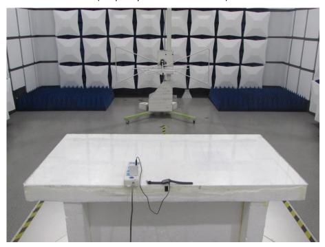
RADIATED EMISSION TEST (Frequency above 1GHz)
