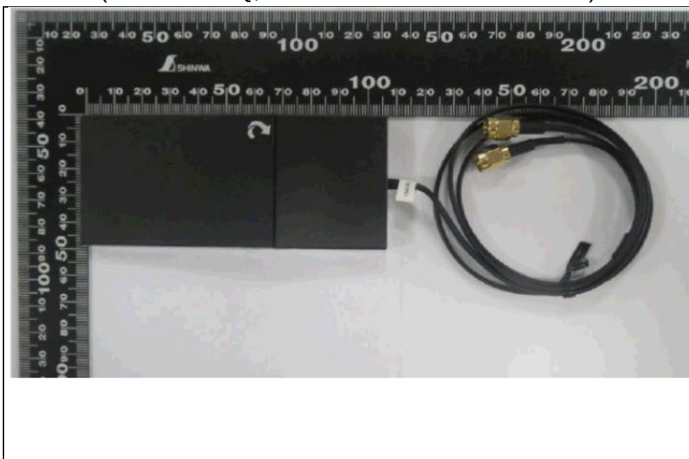
Antenna set 2 (Brand : INPAQ, Model : DAM-I6-H-DB-800-10-17)
