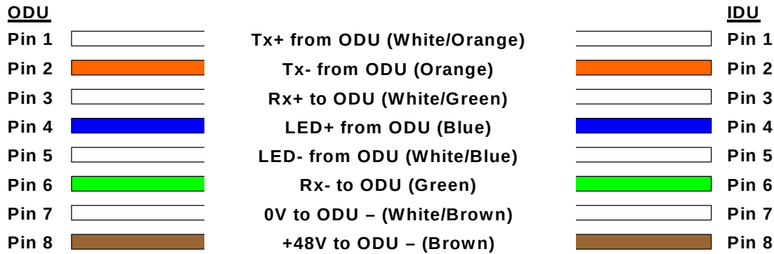
Figure 33 ODU to IDU Connection Diagram
