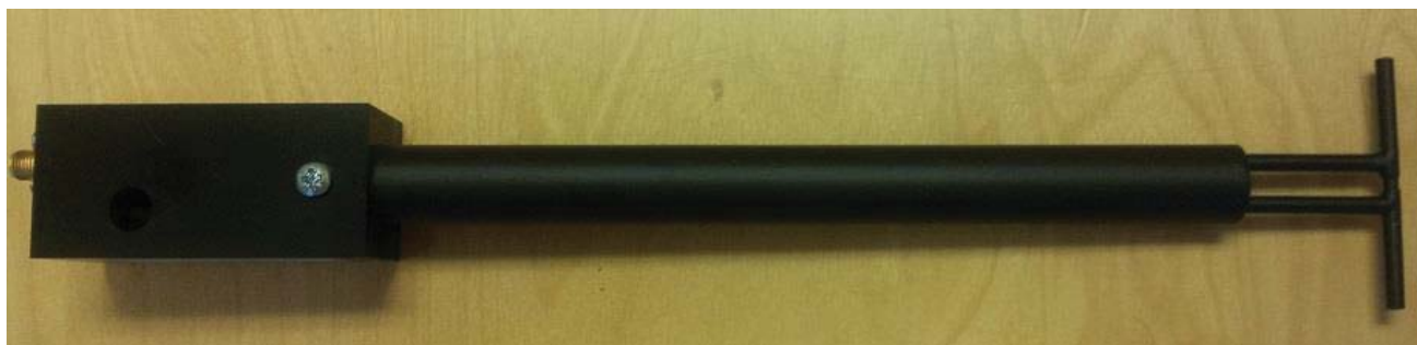
Figure 1 – MVG COMOSAR Validation Dipole
