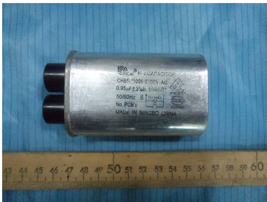
EUT – H.V. Capacitor View
