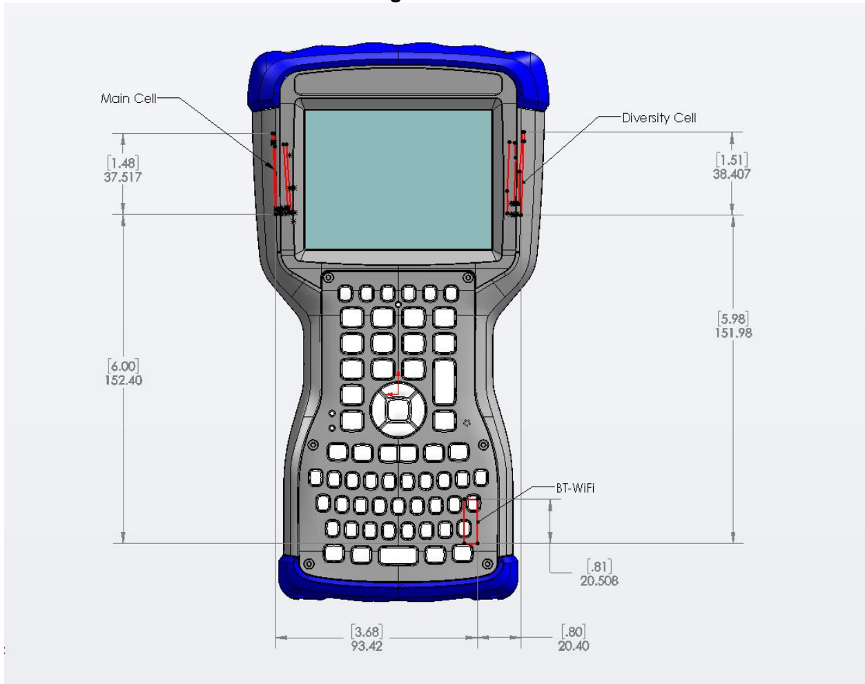
Figure 9.1 SAR Location Diagram of Antenna Distances
