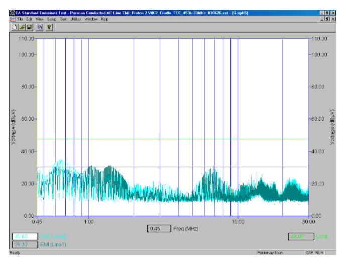
The Handheld was connected to the Docking/Charging Cradle in battery charge mode. The Docking/Charging Cradle data cable was connected to the support PC and to the AC Adapter. The ac input to the AC Adapter was 120 volts, 60 Hz
