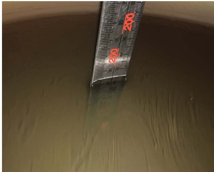
Liquid depth for SAR Measurement
