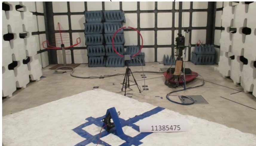
RADIATED BACK PHOTO (BELOW 30MHz)
