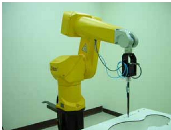
Fig. 5.2 Probe setup on robot
