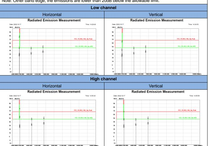
Remark: The emissions for frequency above 18GHz are attenuated 20dB below the limit, it does not record in report.
