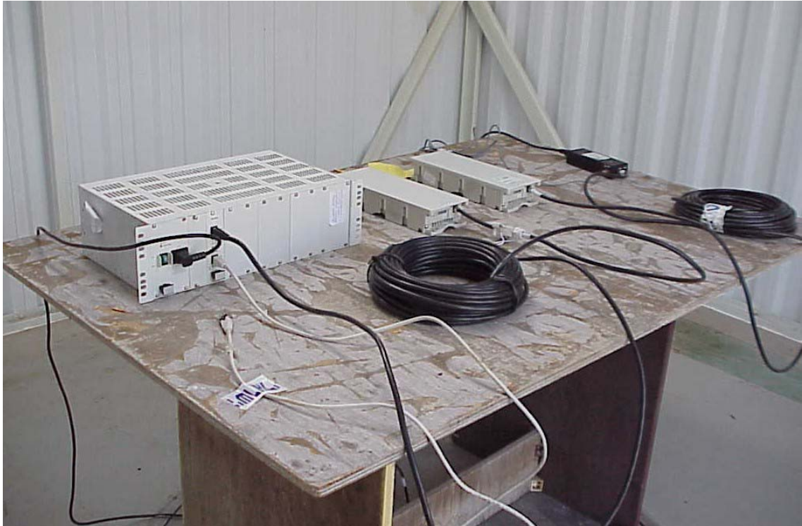
Photo# 4. Radiated emission open site test
