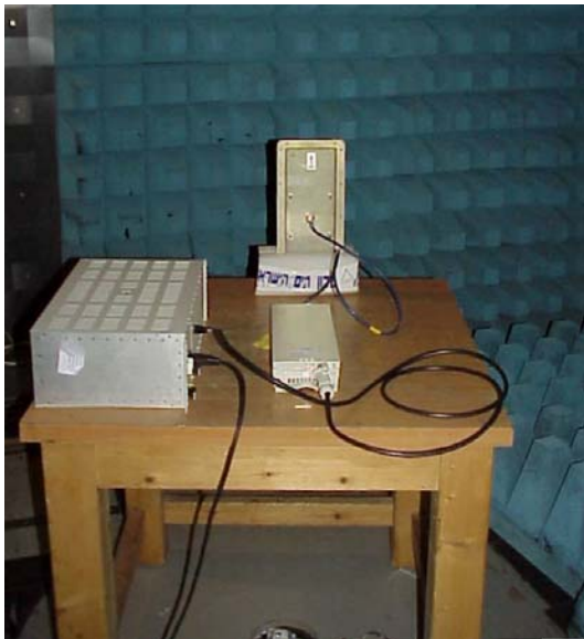
Photo# 5. Radiated spurious emission test. Antenna P/N AN1152
