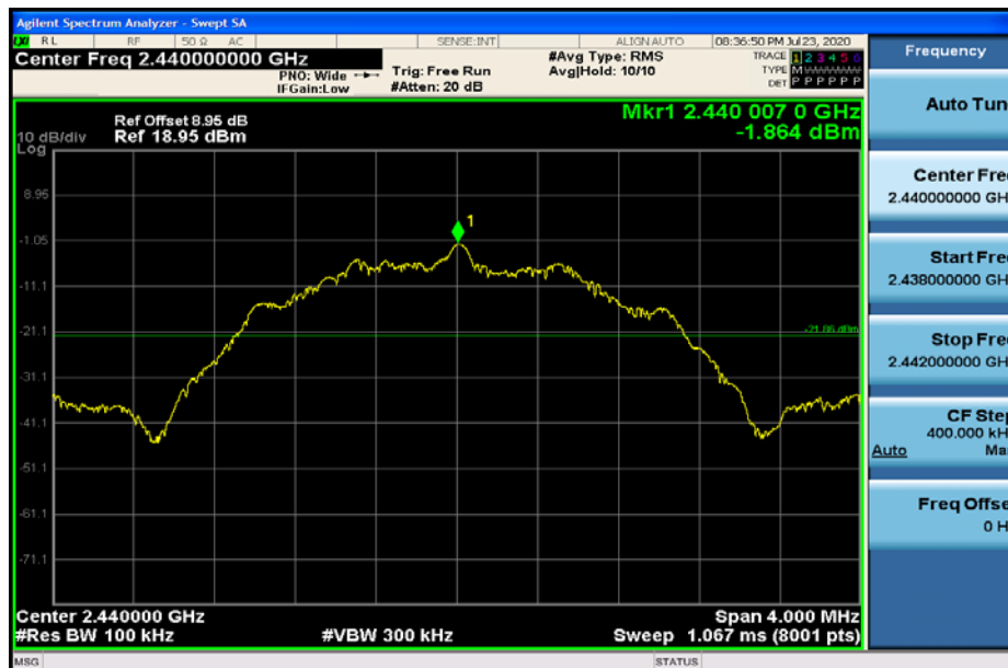
RF Conducted Spurious Emissions_BLE_2440(2M Rate)
