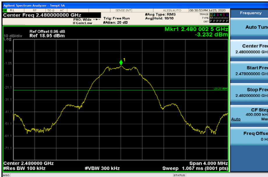
RF Conducted Spurious Emissions_BLE_2480(1M Rate)
