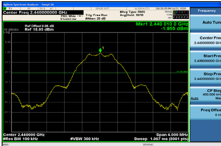
RF Conducted Spurious Emissions_BLE_2440(1M Rate)
