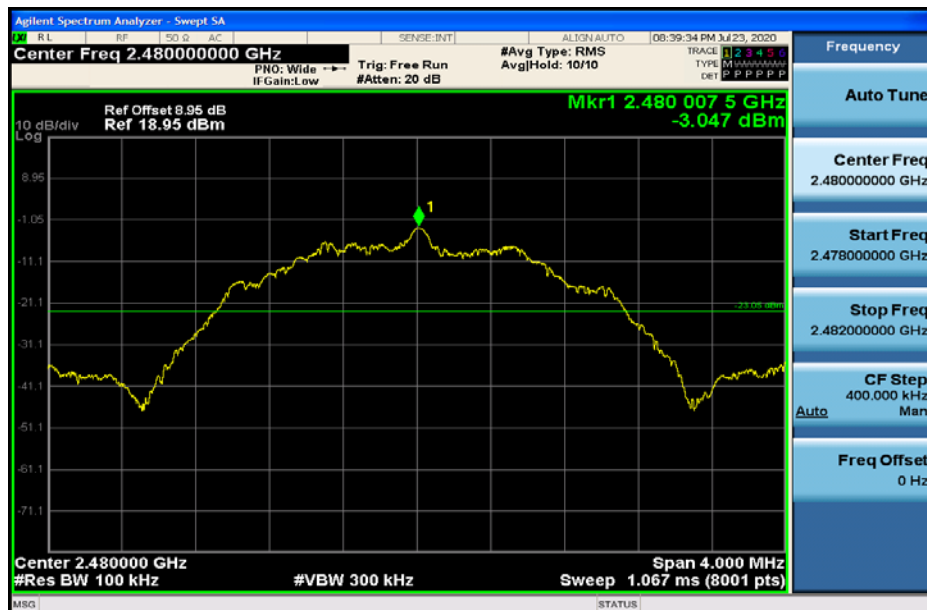
RF Conducted Spurious Emissions_BLE_2480(2M Rate)
