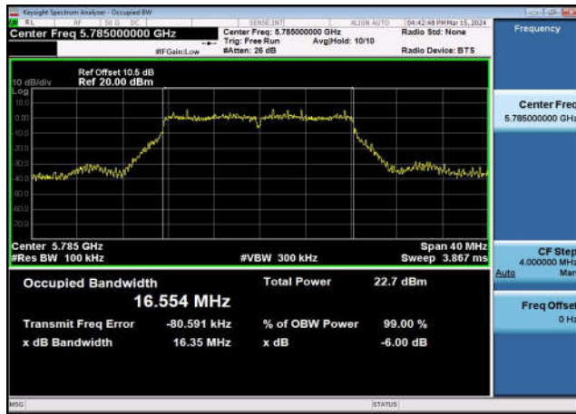
U-NII-3 6dB Bandwidth-802.11a(20MHz) ,5785MHz,Ant1
