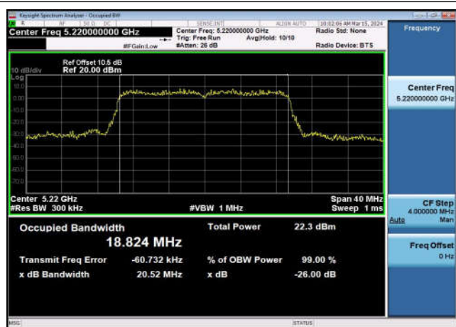
U-NII-1 99%&26dB Bandwidth-802.11ax(20MHz) ,5220MHz,Ant1
