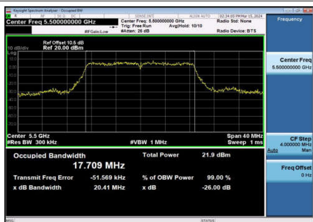
U-NII-2c 99%&26dB Bandwidth-802.11n(20MHz) ,5700MHz,Ant1
