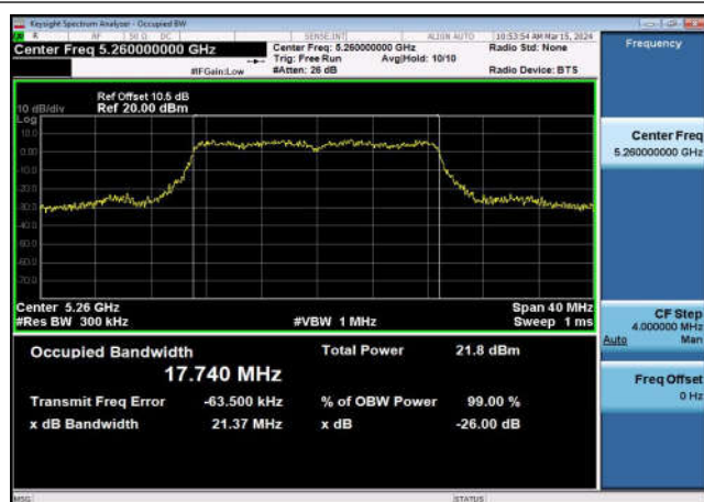
U-NII-2a 99%&26dB Bandwidth-802.11n(20MHz) ,5320MHz,Ant1
