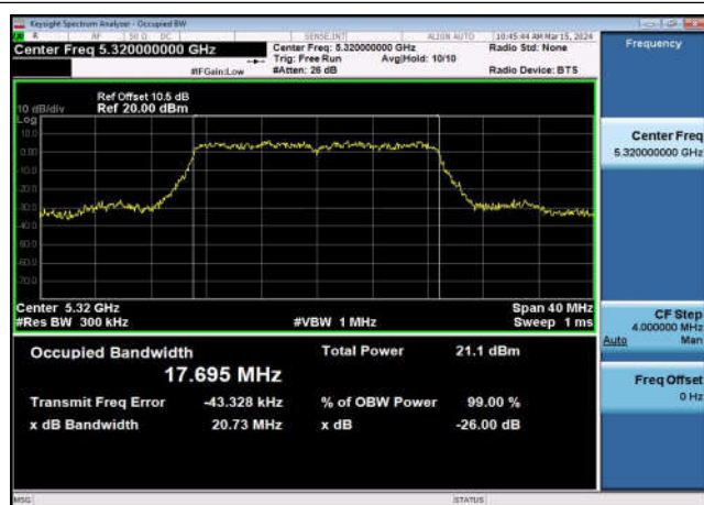
U-NII-2a 99%&26dB Bandwidth-802.11a(20MHz) ,5300MHz,Ant1
