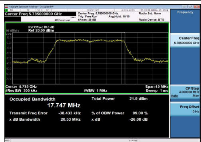
U-NII-3 99%&26dB Bandwidth-802.11ax(20MHz) ,5745MHz,Ant1
