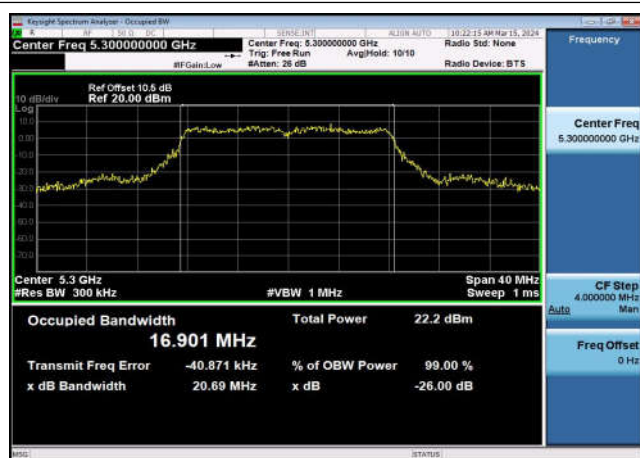
U-NII-2a 99%&26dB Bandwidth-802.11a(20MHz) ,5300MHz,Ant1
