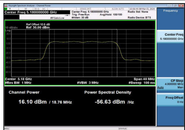
U-NII-1 Output Power-802.11ax(20MHz) ,5240MHz,Ant1
