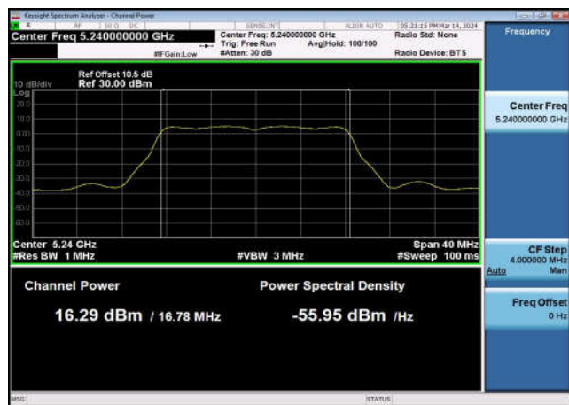
U-NII-1 Output Power-802.11a(20MHz) ,5240MHz,Ant1
