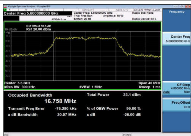
U-NII-2c 99%&26dB Bandwidth-802.11a(20MHz) ,5600MHz,Ant1
