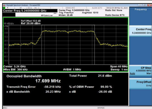
U-NII-1 99%&26dB Bandwidth-802.11ax(20MHz) ,5220MHz,Ant1
