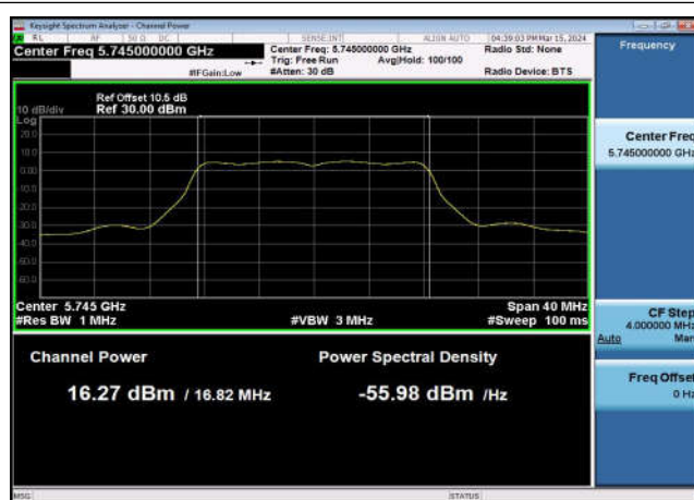
U-NII-3 Output Power-802.11a(20MHz) ,5825MHz,Ant1
