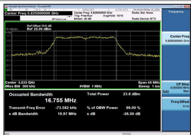
U-NII-3 99%&26dB Bandwidth-802.11a(20MHz) ,5825MHz,Ant1
