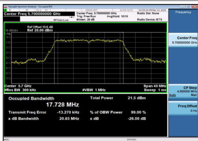
U-NII-2c 99%&26dB Bandwidth-802.11a(20MHz) ,5600MHz,Ant1
