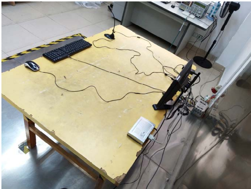
Conducted Emission Test Setup Side View
