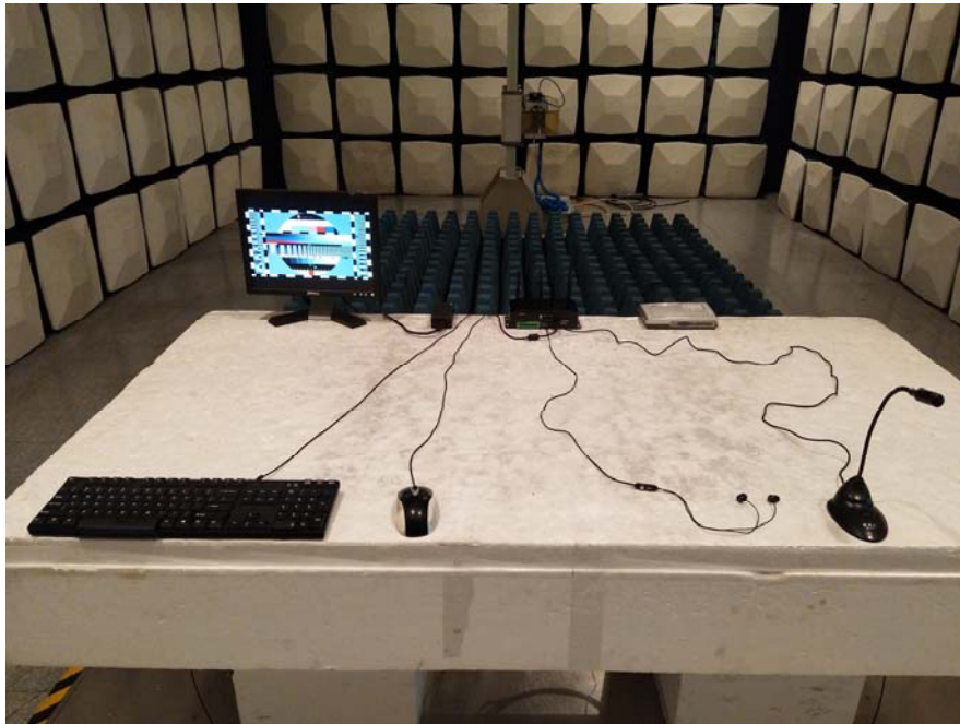
Radiated Disturbance Test Setup Front View (Above 1GHz)
