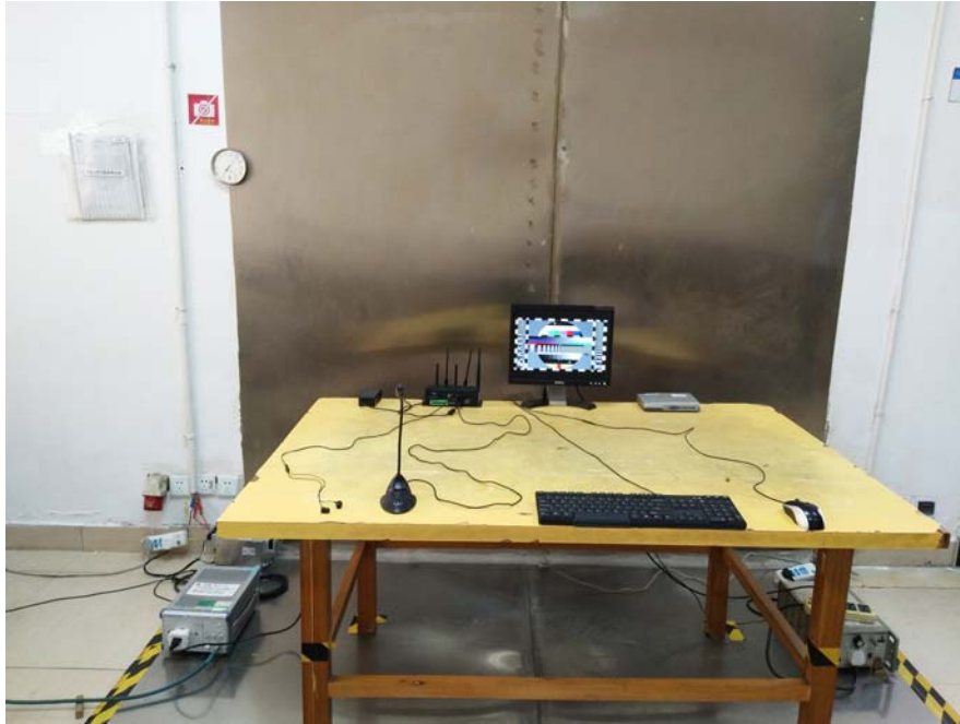
Conducted Emission Test Setup Side View
