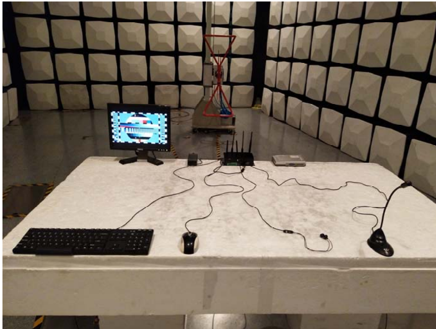
Radiated Disturbance Test Setup Front View (Below 1GHz)
