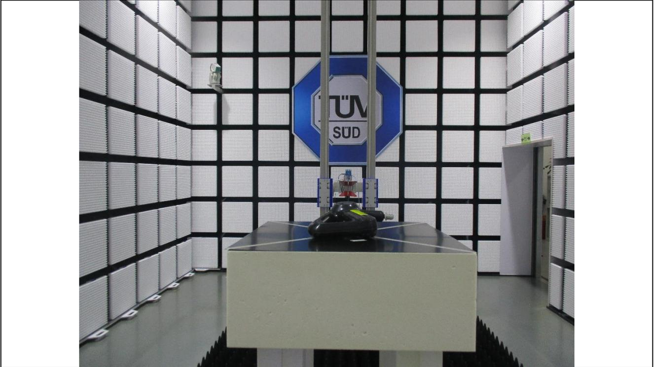
Radiated Emission test (Above 18GHz)
