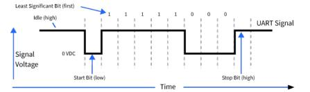
You can configure the UART baud rate, parity, and stop bits settings on the device with the **BD**, **NB**, and **SB** commands respectively. For more information, see <u>Serial interfacing commands</u>.
