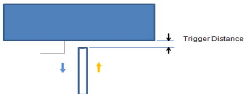
Picture: Proximity sensor triggering distances assessment (Bottom)
