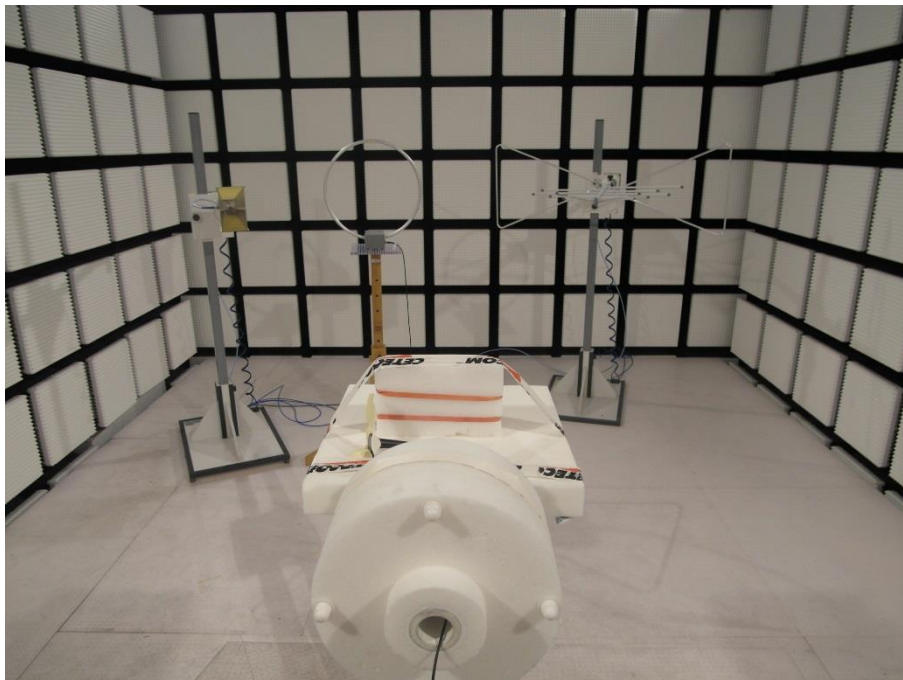
Photo 5: EUT at the anechoic chamber
