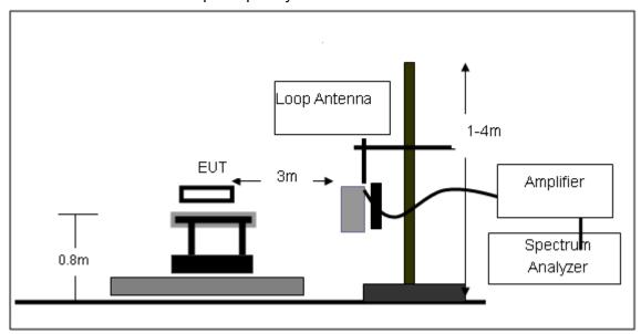
(B) Radiated Emission Test-Up Frequency 30MHz~1GHz
