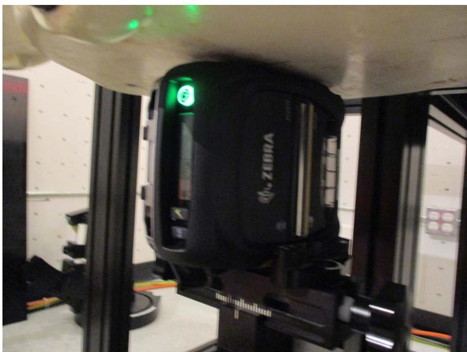
**1.3 EUT Bottom Side handheld configuration touch to the Flat Phantom Setup Photo – Right Side**
