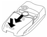
Place the SIM card in front of the slot with the contact surface facing downwards. Then press the
