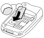
Insert the battery into the phone <sup>4</sup>, then press it downwards <sup>5</sup> until it engages.
