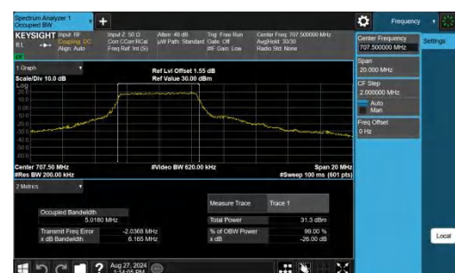
Band12-10MHz-16QAM-23095-27RB#0-PASS
