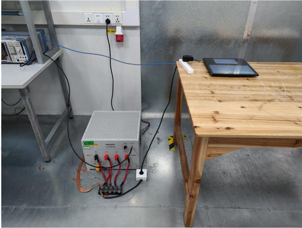
Photo of Power Line Conducted Emission Test
