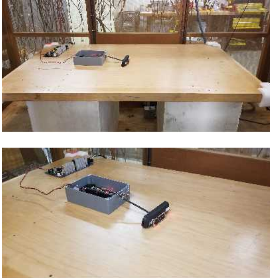
Figure 6: Conducted Emissions Test Setup Photograph(s).
