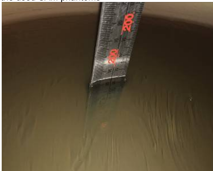
Liquid depth for SAR Measurement
