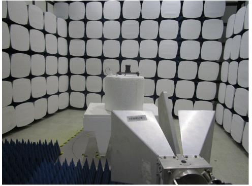
1.3 Radiated Spurious Emissions Test Setup
