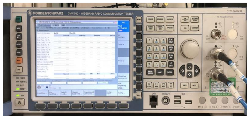
CMW 500 (2G/3G/4G Test Equipment)
