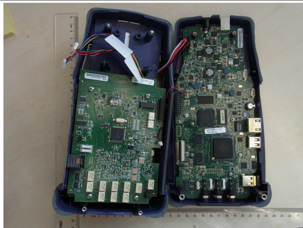
Figure 14: Internal view CSC-TPSVW-CU, SCTPS-AB-CU
