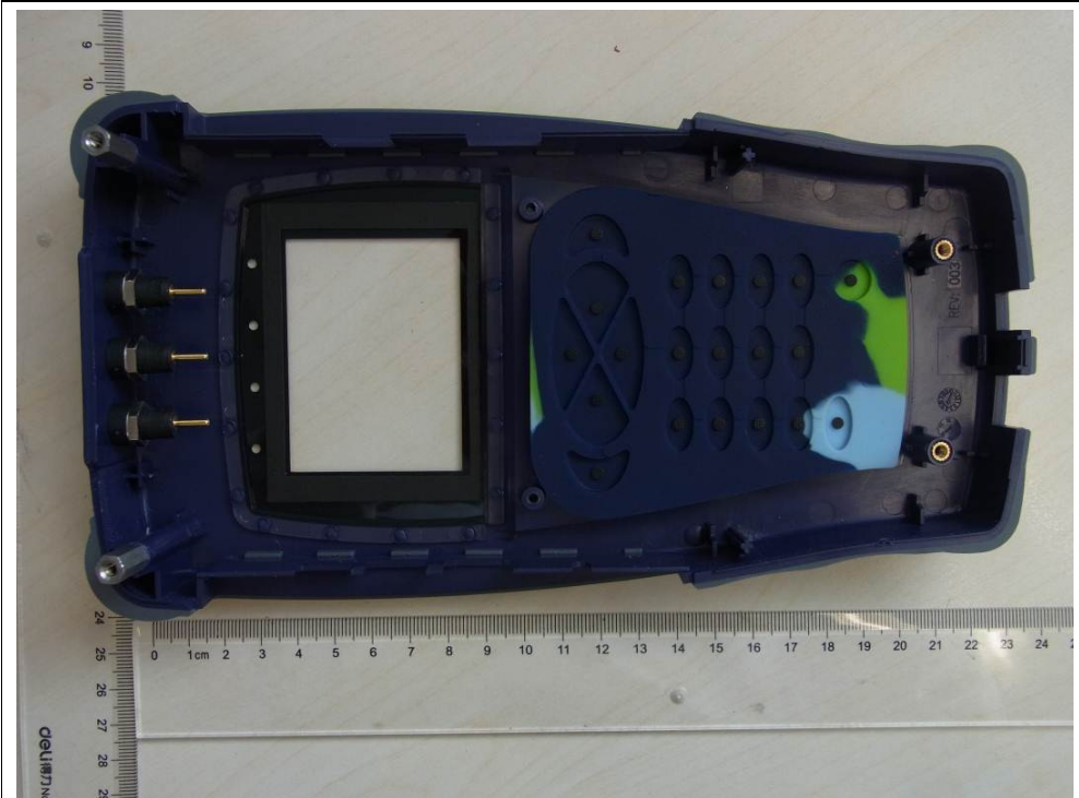
Figure 17: Internal view top enclosure
