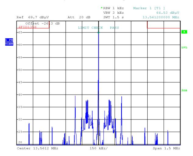
The values of the plot are extrapolated to a measurement distance of 3 m. (Calculated limit @ 3m: 124  $dB\mu V/m$ )
