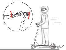
4. Release the accelerator and the kinetic energy recovery system (KERS) initiates automatically to brake slowly; And squeeze the brake lever for a sudden brake.
