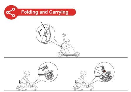
Make sure that the scooter's turned off. To fold, unlock the folding mechanism, and bend the handlebar stem to hook the buckle on the rear fender. To open, press the bell trigger to remove from the buckle, erect the handlebar and lock the folding structure.
