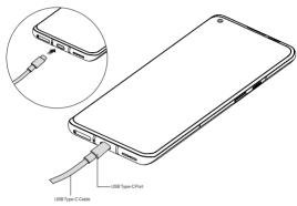
Connect the USB Type-C cable to the USB port on your device, which is located on the lower center of your phone.
