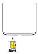
Please use the SIM Tray Ejector (found in the box) to remove the SIM tray from the device and insert Nano SIM cards in the tray.
