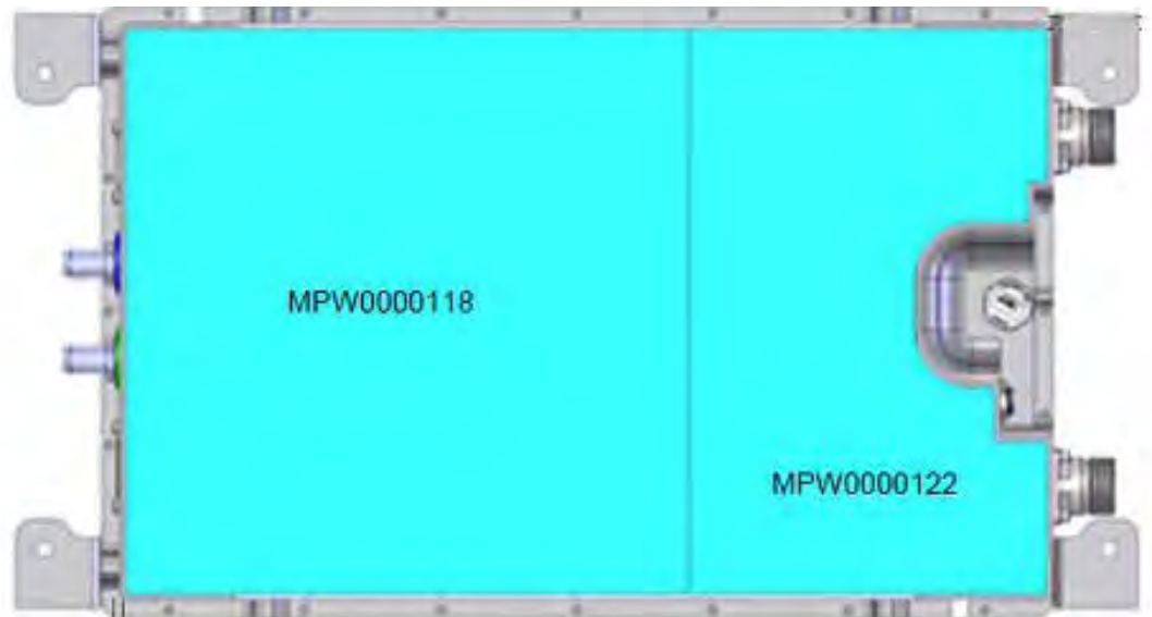
Figure 4-7. KRFU Thermal Pads
