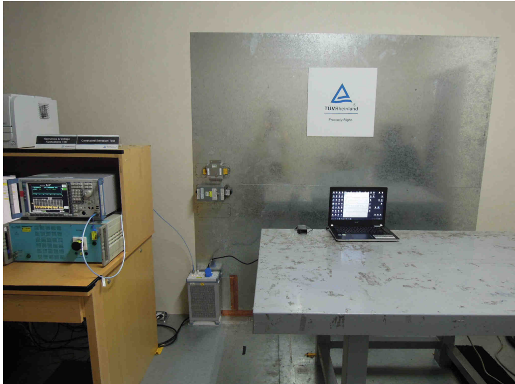
Photograph 6: Set-up for for Mains Conducted testing Front
