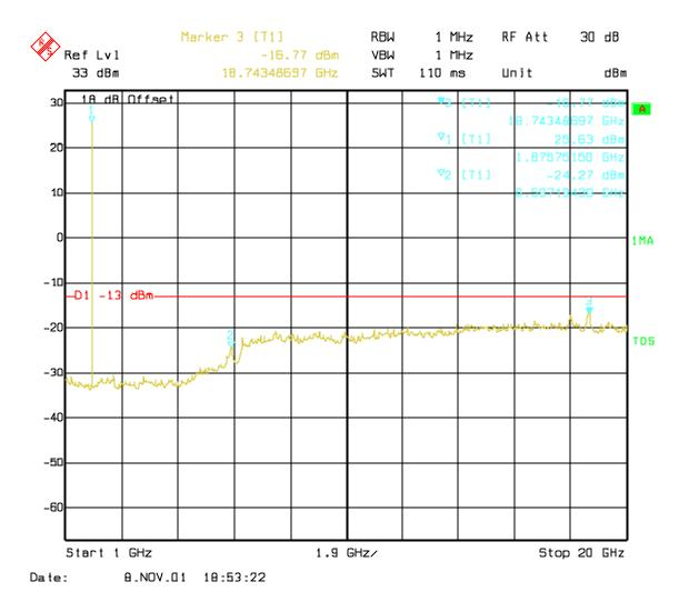
NOTE: Frequency resolution is not fine enough to show the exact frequency of the carrier, refer to plots under EIRP.
