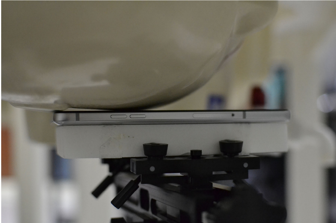
SAR Test Setup Photo 1 – Right Cheek
