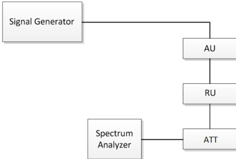
Fig.3. Input-versus-output Signal Comparison
