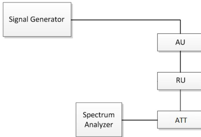
Fig.6. Out-of-band/out-of-block (including intermodulation) Emissions and Spurious
