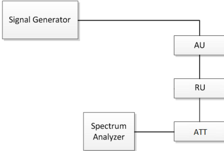
Fig.2. Out-of-band Rejection
