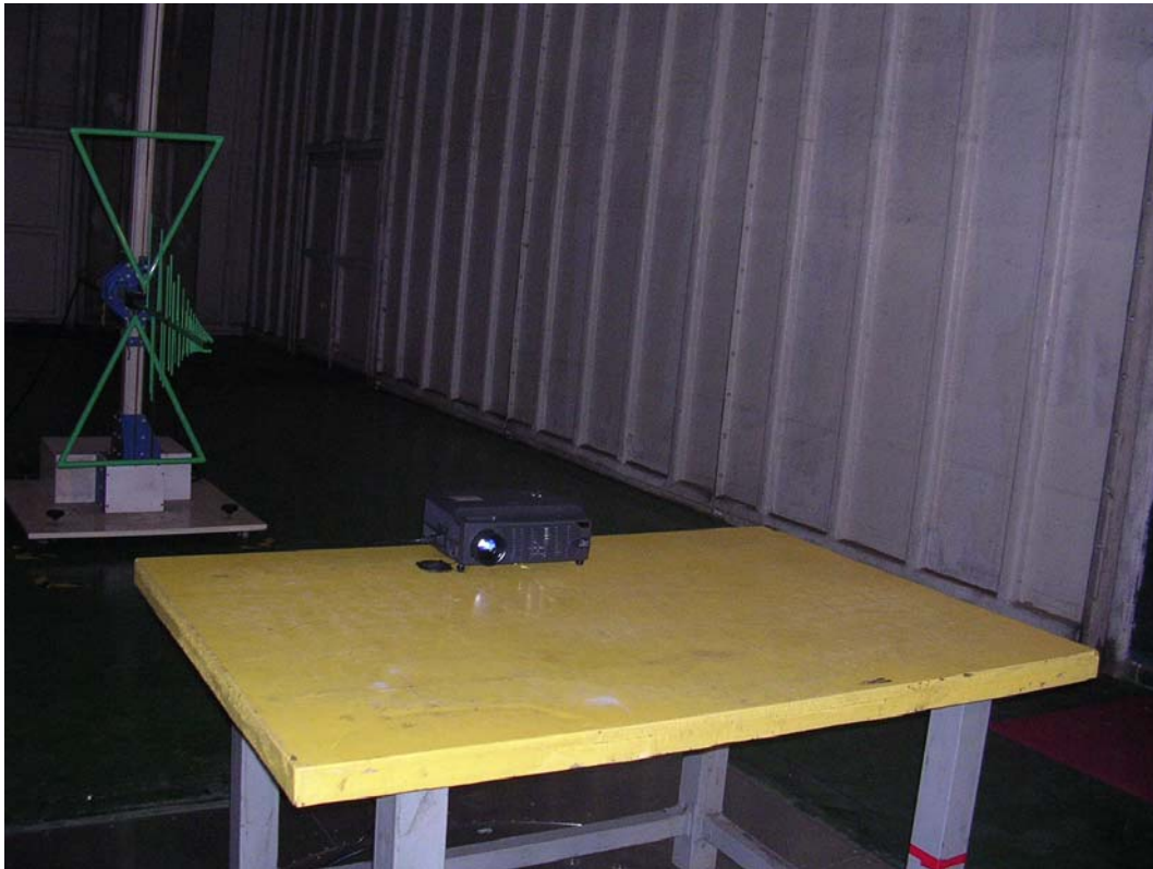
Front View of Radiated Test
