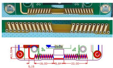
Antenna transmission frequency: 433.925MHz Antenna type: PCB antenna Antenna Gain: -12.12 dBi
